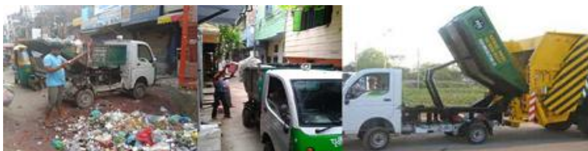
Figure-6: Direct transfer of mixed waste from auto-tippers to tipper-trucks
