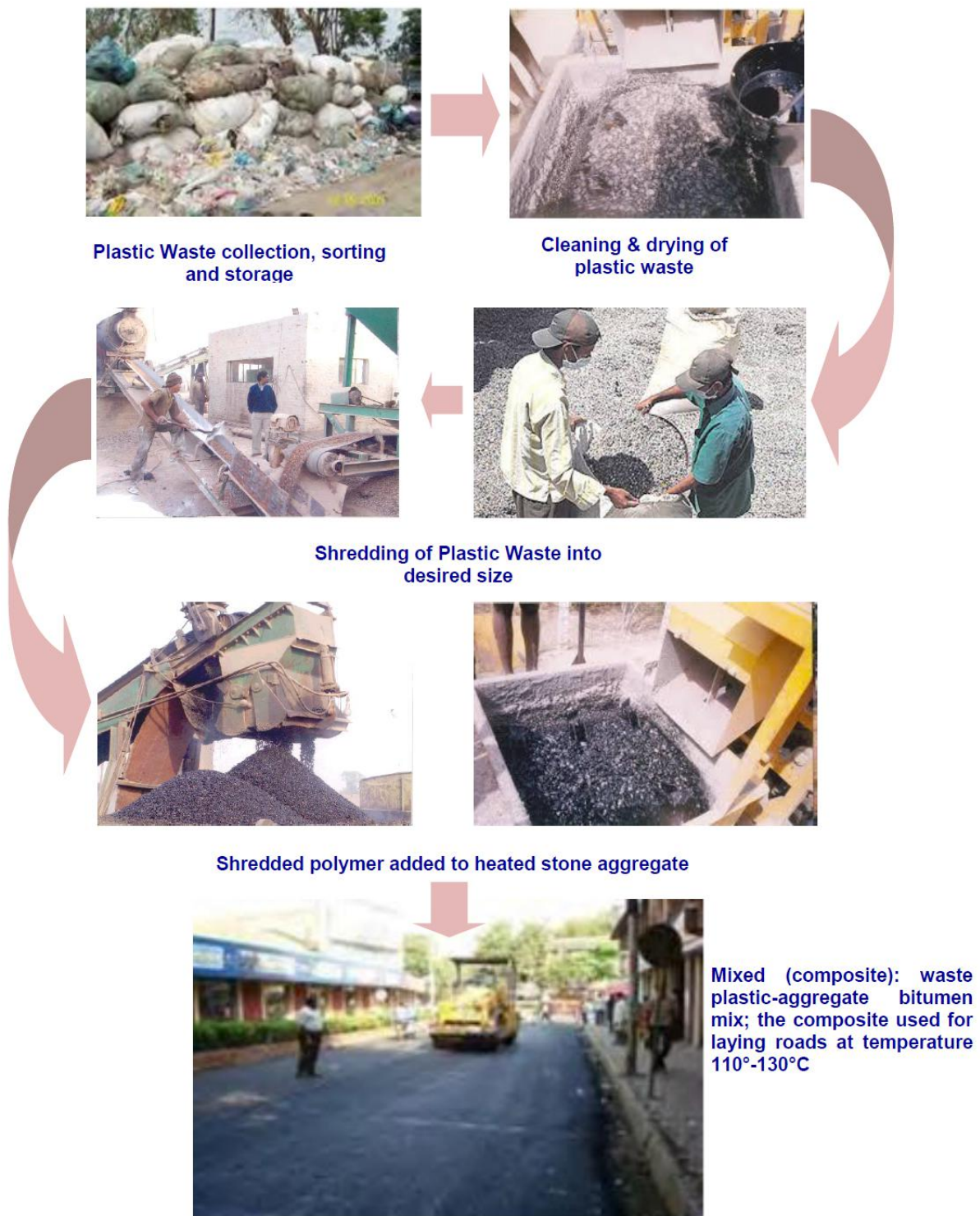
Figure-104: Process Diagram for Laying Road using Waste Plastic-aggregate Bitumen Mix
